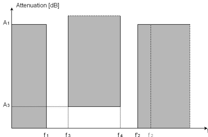
Stop-bands:  $A_1 = 30 \text{ dB}$ ,  $f_1 = 440 \text{ kHz}$ ,  $f'_2 = 470.4545 \text{ kHz}$
