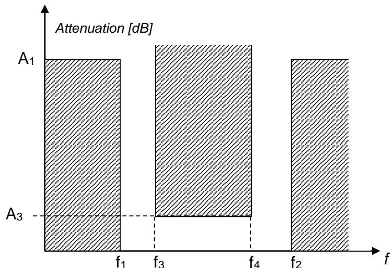
Stop-bands:  $A_1 = 30 \text{ dB}$ ,  $f_1 = 440 \text{ kHz}$ ,  $f_2 = 475 \text{ kHz}$
